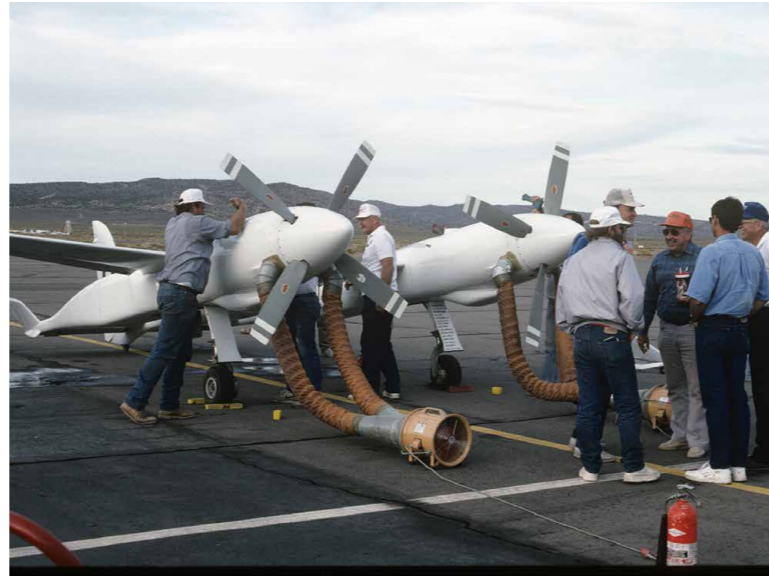
Pond Racer's methanol-fueled engines needed meticulous care. Among other headaches: Immediately upon shutdown, the crew had to hurry to attach cool-air blowers to each engine.
